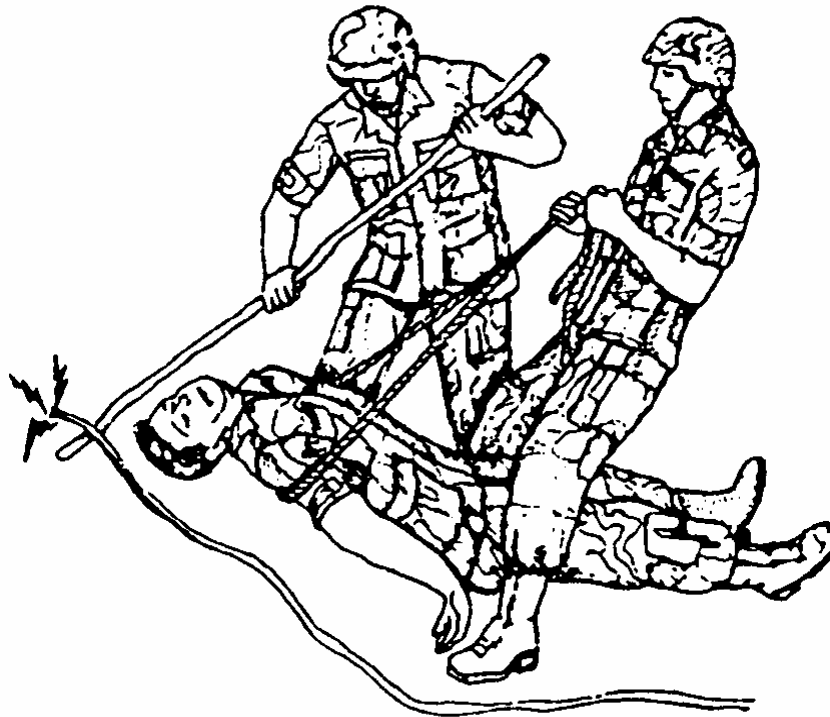
Figure 6-7. Removing an electrical wire beneath a casualty.
